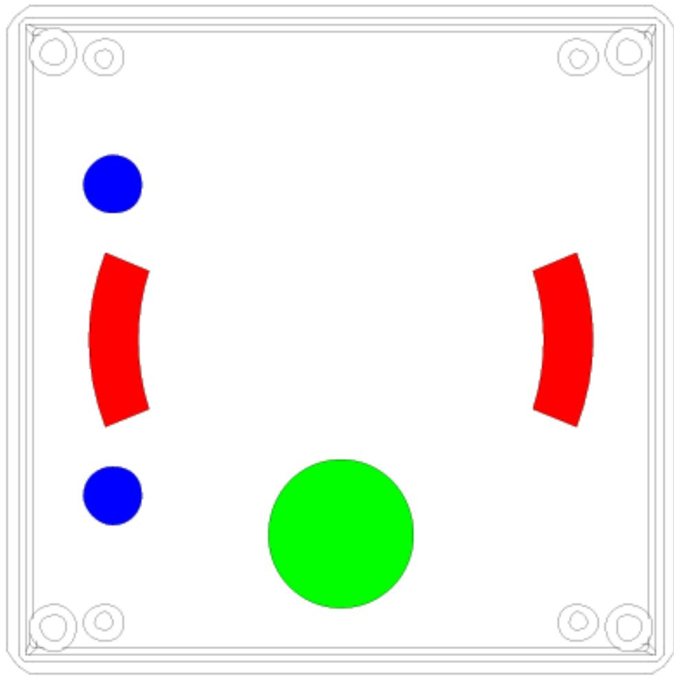
The colour green indicates the opening intended for the communication and power wiring.
